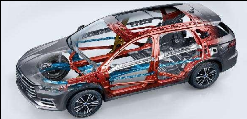
The body stiffness is 21872 N·m, which can strengthen safety protection in crash reduction and deformation.
