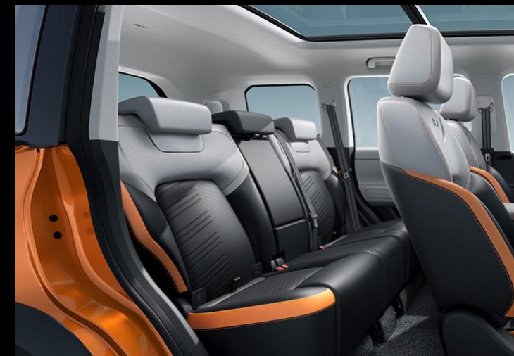
The rear seat angles adjustment support 26 degrees adjustment (front 16°, rear 10°)
