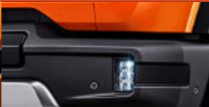
Segmented LED fog light With steering assist function
